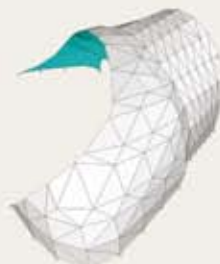
AREA ELEMENT MODEL The inflatable structure is made up of a combination of tube elements and skin elements. This computer model shows the distribution of the skin elements.
