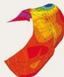
STRESS ANALYSIS MODEL The final image shows the stress distribution within the diaphragm shell. Purple and red denote areas of low stress and the blues and greens show the areas of high stress.
